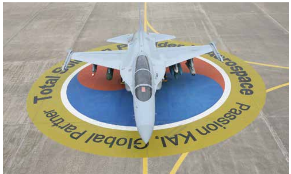
FA-50 fighter aircraft ground display with various weapons. AIM-9 Sidewinder air-to-air missiles, AGM-65 Maverick air-to-surface missiles, Mk-82 500lb bombs, SFW WCMD CBU-105 smart cluster bomb, and JDAM GBU-38/B 500lb bomb.
